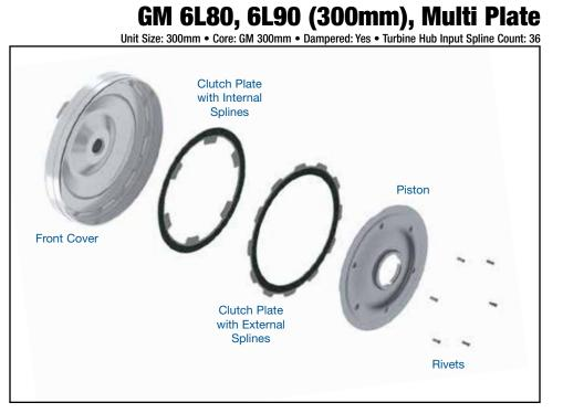
**NOTE:** Do NOT use the force of peening the rivet to clamp the pads together and against the piston. It is important to use an alternate clamping force to contact both the rivet pads and the piston before installing rivets.
