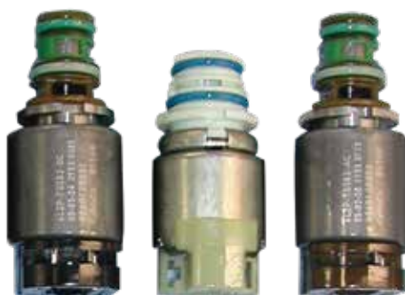
6R80 (2009) Black & brown connectors in most locations. SSE solenoid has clear connector and white snout 2009-2011
