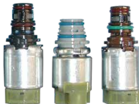
6R80 (2010-Later), 6R100 Clear connectors with black & brown snouts in most locations. SSE solenoid has clear connector and grey snout. Solenoids are banded (1-5) for flow rate.
