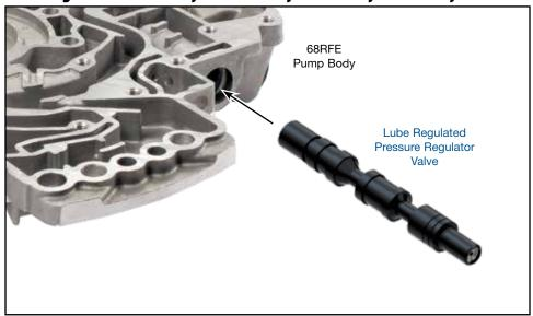
NOTE! Check casting wall at the pressure regulator valve between the line and lube/converter circuits. If a hole has been drilled in this wall, it must be plugged shut to receive full benefits from this valve.
