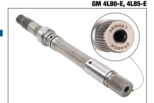
**NOTE:** Eliminating the undercut between splines and step that seats against the overdrive carrier makes the Sonnax shaft considerably stronger in this area that commonly fails (**Figure 1**).
