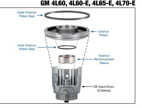
Use Stamped Steel Forward Piston This kit must be used with a '97-later stamped steel forward piston or the aluminum piston in Sonnax forward sleeve kit 77733-52K. It cannot be used with '96-earlier OE cast aluminum forward piston or older Sonnax billet forward piston 77764-01.
