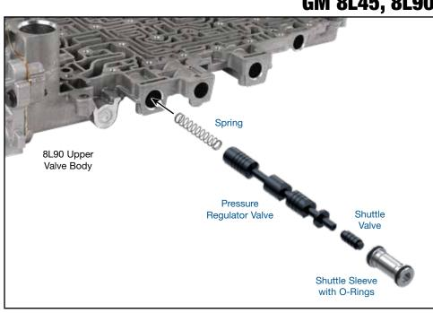
CAUTION! Sonnax shuttle valve assembly included in this kit should only be used in combination with Sonnax pressure regulator valve. Linear dimensions have been altered, and mixing Sonnax and OE components could result in drivability issues.
