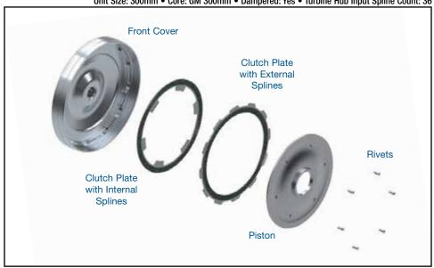
**NOTE:** Do NOT use the force of peening the rivet to clamp the pads together and against the piston. It is important to use an alternate clamping force to contact both the rivet pads and the piston before installing rivets.
