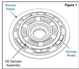
f. If cracks are found replace this part with Sonnax GM-DA-18 spring retainer plate.
