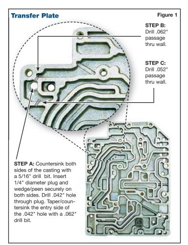
b. On the transfer plate (**Figure 1**), drill a .062" hole through the indicated wall. This will connect the line pressure circuit to the differential lube circuit.
