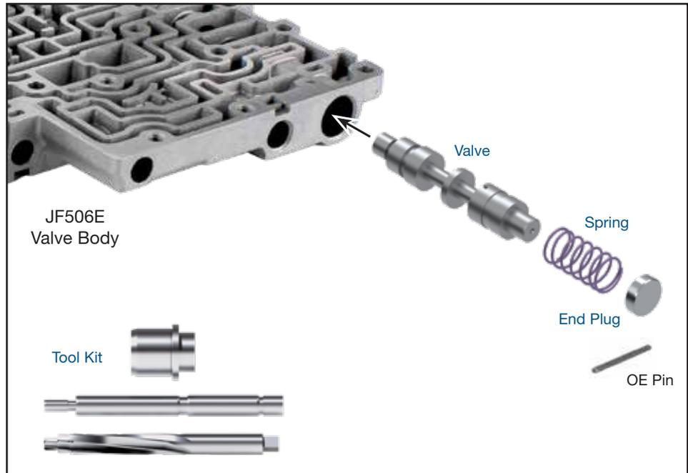
**NOTE:** Sonnax “F-Tool” kits designed to service a specific bore require the VB-FIX, a self-aligning valve body reaming fixture. More information and instructions can be found online at [www.sonnax.com](http://www.sonnax.com).
