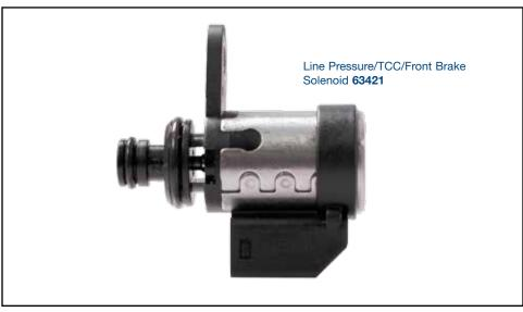
**NOTE:** Solenoids may be difficult to remove from valve body. Carefully twisting a flat-blade screwdriver between retainer bracket and valve body can ease solenoid removal. Alternately, a punch inserted from bottom of channel plate can be used to lightly tap solenoid snout outward.
