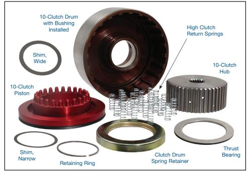
To ensure maximum clutch plate engagement with the hub splines, Sonnax 10-clutch hubs are manufactured with a minimal chamfer at the indicated area. When using non-Sonnax flanges, you must check the clearance between the chamfer on the hub and the sun gear flange to ensure there is adequate clearance. If more clearance is needed, machine a greater chamfer on the hub as necessary.
