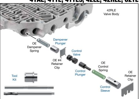
**CAUTION:** For 40 and 41 series transmissions, this kit CANNOT be used in early units that have #33 separator plates. Kit can only be used in later designs that have a #4 retainer clip in the TCC control valve bore (main illustration).
