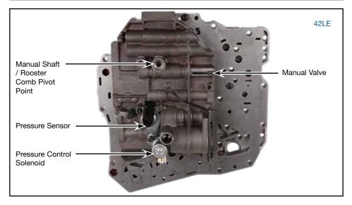
Mishandling or shipping Sonnax 41TE VLP remanufactured valve body **CHR400** or 42LE VLP remanufactured valve body **CHR402** with the manual shaft/rooster comb attached to the valve body can cause the manual valve bore to be crushed enough to jam the manual valve in the bore.
