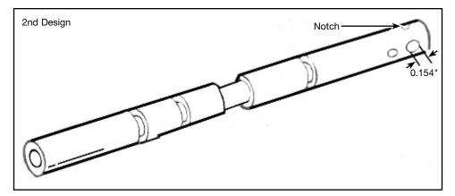
First ('91-early '92) or second design (late '92-later) manual valves for the Saturn TAAT are used with the flat manual valve link. They should be installed with flat (first design) or notch (second design) facing up.
