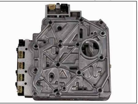
Whenever a valve body is installed into an 096, 097, 098, 01M, 01N or 01P transmission, the internal manual valve linkage must be adjusted to sync up the manual valve with the rooster comb and external linkage.
