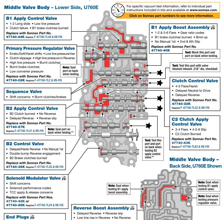
\*\*These two passages are connected. The mat will provide the seal for the middle valve body. upper side. The passage indicated (\*\*) will also need to be sealed to vacuum test the circuit.
