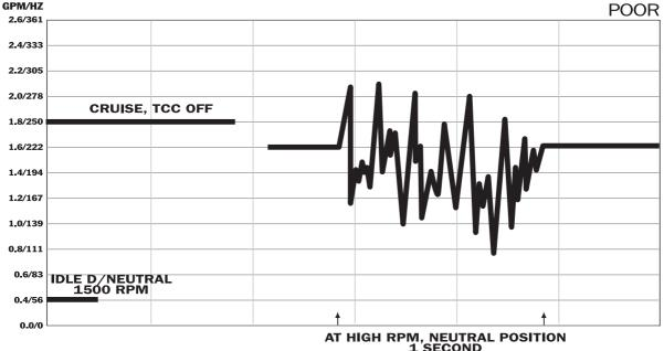
**Condition:** Slip bump forward, TCC pulling down, engine stall, delayed engagements, falling out of gear.
