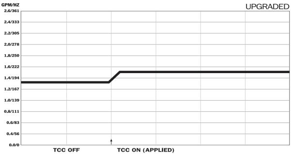
**Correction:** Improved lockup with Sonnax Bypass Control Sleeve & Plunger **96206-01K**.
