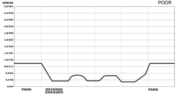
**Condition:** Poor pump output, line pressure and cooler flow cannot be maintained. **Correction:** Pump must be rebuilt.
