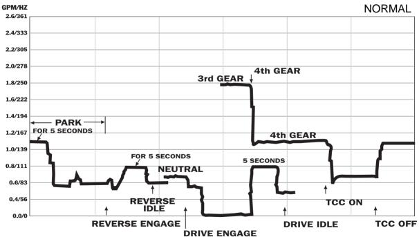
Notes: Park cooler flow was stable for 5 seconds at .8, then goes up for 5 seconds at 1.1, then down to .6. Reverse and neutral also go up for 5 seconds and then settle down.
