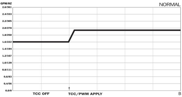
**Condition:** Improved TCC transition with Sonnax Bypass Clutch Control Sleeve & Plunger Valve **76948-04K**.
