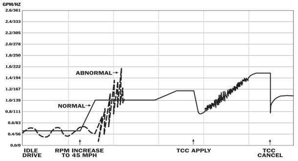
**Condition:** Weak pump. Note low flow idle drive oscillation. Low oil level and/or filter gasket sucking air on acceleration.
