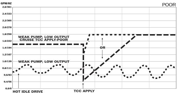
**Correction:** A good TCC should be quick and sharp rise to 1.8 to 2.1 gpm.
