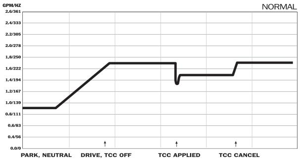
Notes: Vehicle had repetitive converter failure. TCC came on immediately at 35 mph, which loaded it heavily. Lift foot and TCC would come off. As soon as the throttle touched, TCC reapplied. The Bosch EDC solenoid will cycle a cleaning spike, which affects the flow.
