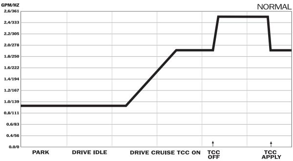
**Condition:** Normal to slightly elevated, TCC drop may be .4 gpm. Non-PWM decrease flow during TCC apply. The key to any unit is an occurrence of a noticeable change.
