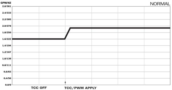
**Condition:** Improved TCC transition with Sonnax Bypass Clutch Control Sleeve & Plunger Valve **76948-04K**.
