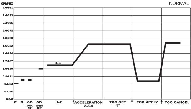
Notes: Flow drops in TCC apply, quick valve action.
