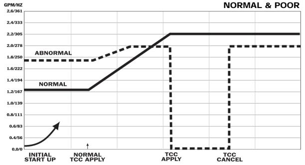
**Condition:** Dotted line is with TCC control valve installed backward.
