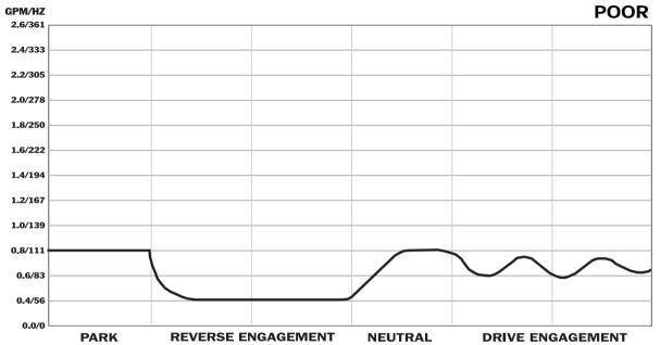
**Condition:** Repeated 3-4 clutch failure, 2nd gear starts when hot due to low AFL psi.
