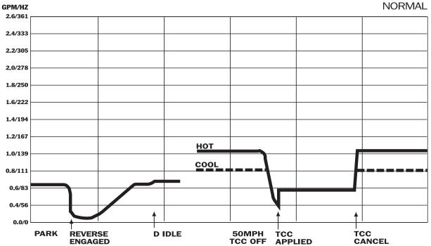
Notes: Very low flush at 45 degrees F, .3 gpm Park, Reverse, Drive. Flow sensitive to rpm and .4-.6 gpm during shift. Unit has been flushed on DCI HOT FLUSH and flowed well.
