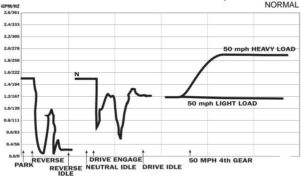
**Notes:** Top is raw frequency data read at the 500 Hz range setting. This captured momentary fluctuation is flow during valve activity. Chart below is how that would appear on SonnaFlow LED readout alone.
