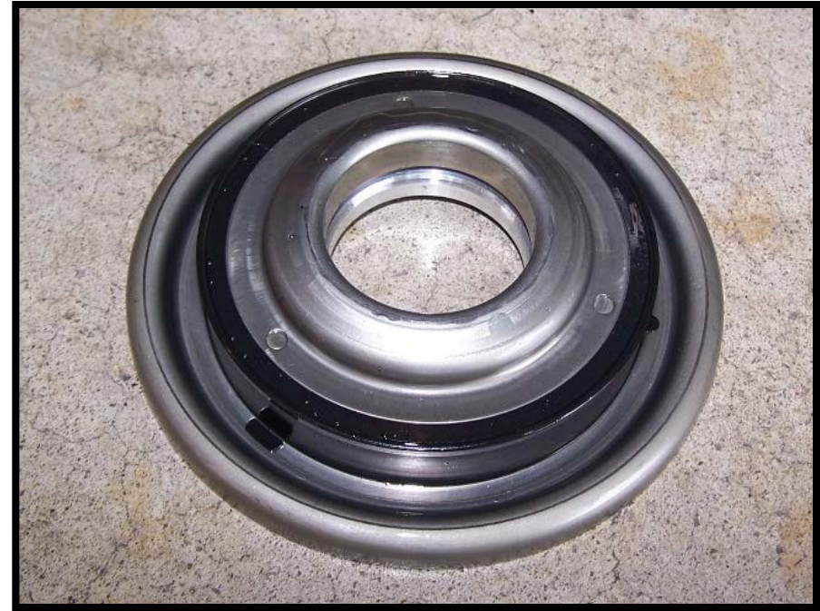
Bottom of the E Clutch Piston (Bonded Side)
